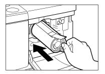
**6** Holding the toner cartridge steady with one hand, firmly and slowly pull the sealing tape tab with the other hand to remove the sealing tape completely. Throw the tape away.
